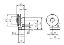
Guide pulley for draw-wire encoder Order code 8.0000.7000.0031
