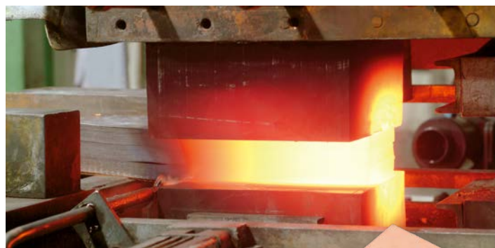
Pressure welding process for copper connectors
