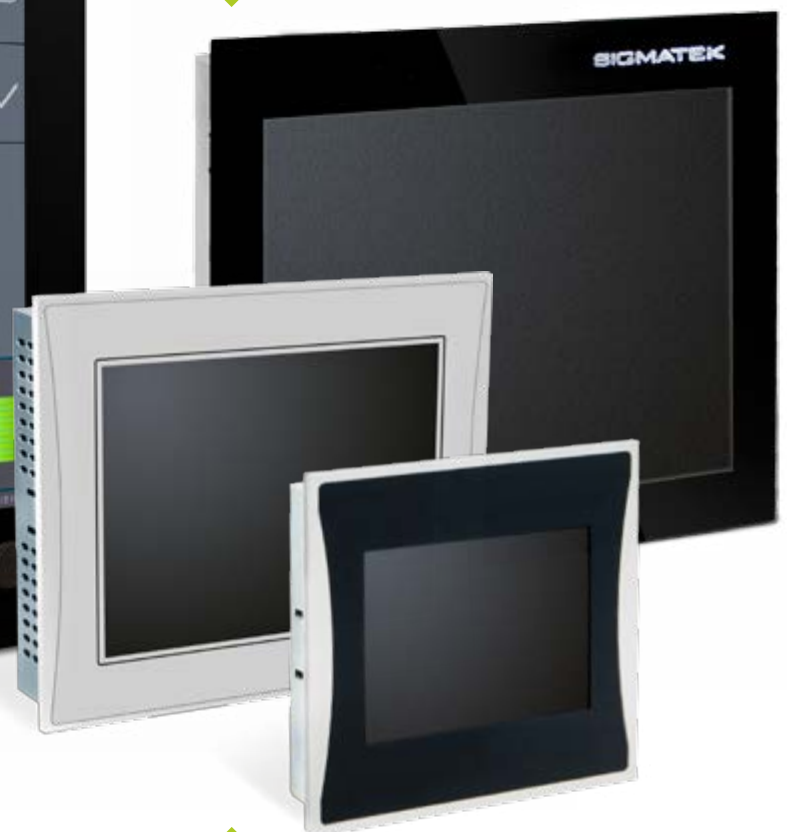
For simple applications, all-in-one control panels from the ETV series are available. Small panels for operating and monitoring are already available from 3.5 inches.
