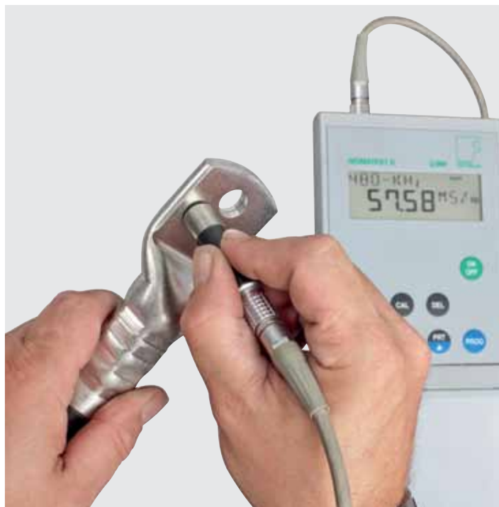
Testing of the conductivity
