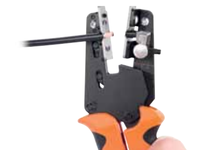
Automatic removal of insulation
