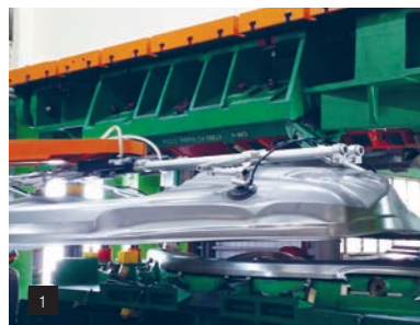
1 2 LEMAX+ vacuum pumps and C-series high-performance suction cups for handling stamped parts.
