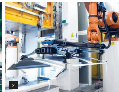
1 2 LEMAX+ vacuum pumps and C-series high-performance suction cups for handling stamped parts.
